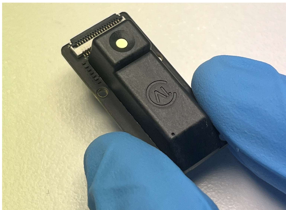
Figure 10: Recommended handling touch points of the CTS module. Gloves should always be worn when handling the sensor
