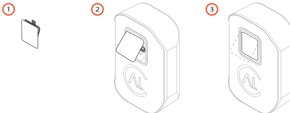
Figure 20 - Installation procedure for the infrared film
